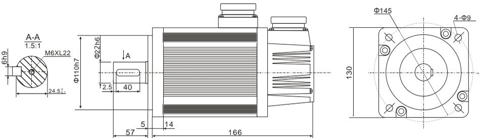
Figure 3.5 1KW (Middle inertia) type Motor installation dimension (Unit: mm)
