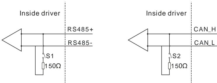
In order to improve reliability of the communication data, both ends of the communication cable should be limited when building CANopen network, that is connecting a termination between CAN\_L and CAN\_H of the servo. The following figure indicates the termination method among E10 Servo Driver and CPU226M-CAN.
