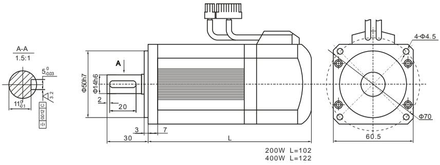
Figure 3.3 200W/400W (Low inertia) type Motor installation dimension (Unit: mm)
