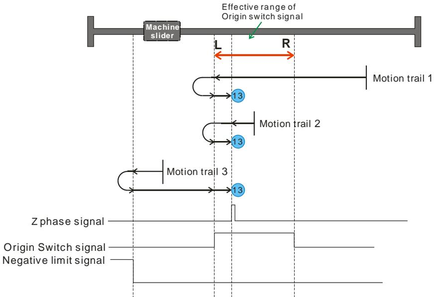
As seen above, machine is moving to the negative limit switch, Z-phase signal is located at right of left edge of the original point signal, which is within the range of original switch.
