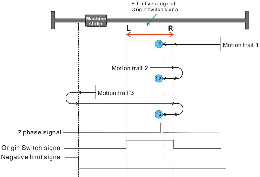
As seen above, machine is moving to the negative limit switch, Z-phase signal is located at left of right edge of the original point signal, which is within the range of original switch.
