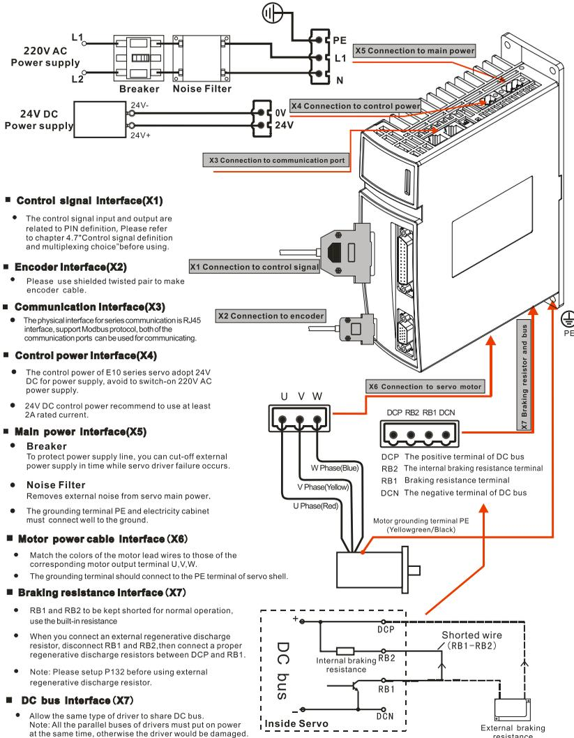
Figure 4.1 External port schematic diagram
