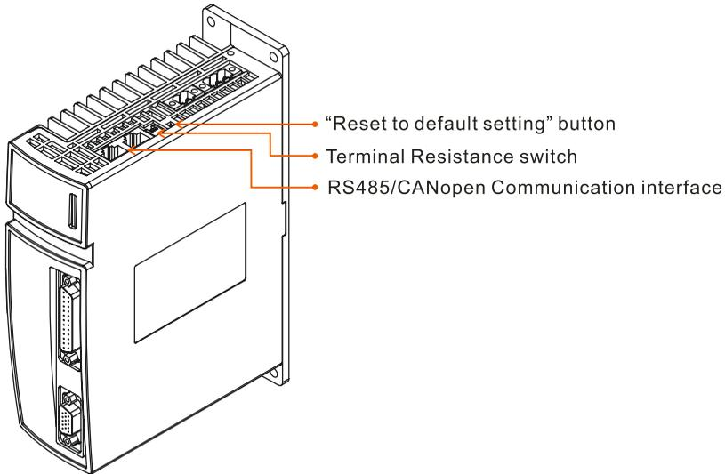
Figure 4.6 The schematic diagram of servo top terminal
