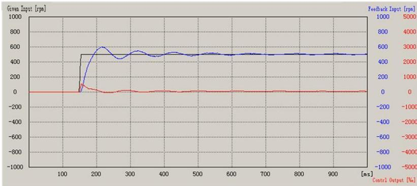
Figure 9.8 The speed loop curve of insufficient integration time of increasing the inertia ratio
