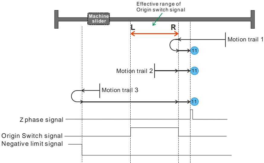
As seen above, machine is moving to the negative limit switch, Z-phase signal is located at right of right edge of the original point signal, which is out of the range of original switch.
