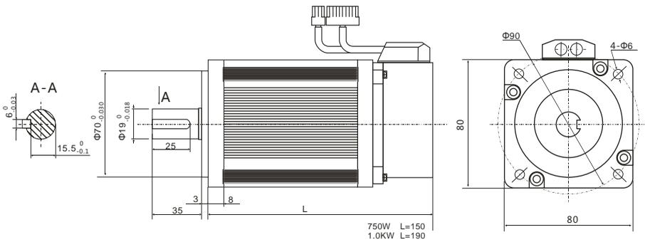
Figure 3.4 750W/1KW (Low inertia) type Motor installation dimension (Unit: mm)
