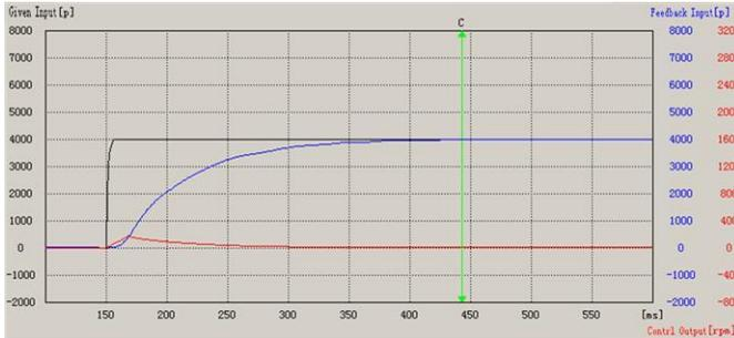
Figure 9.6 The position loop curve at low gain of position loop
