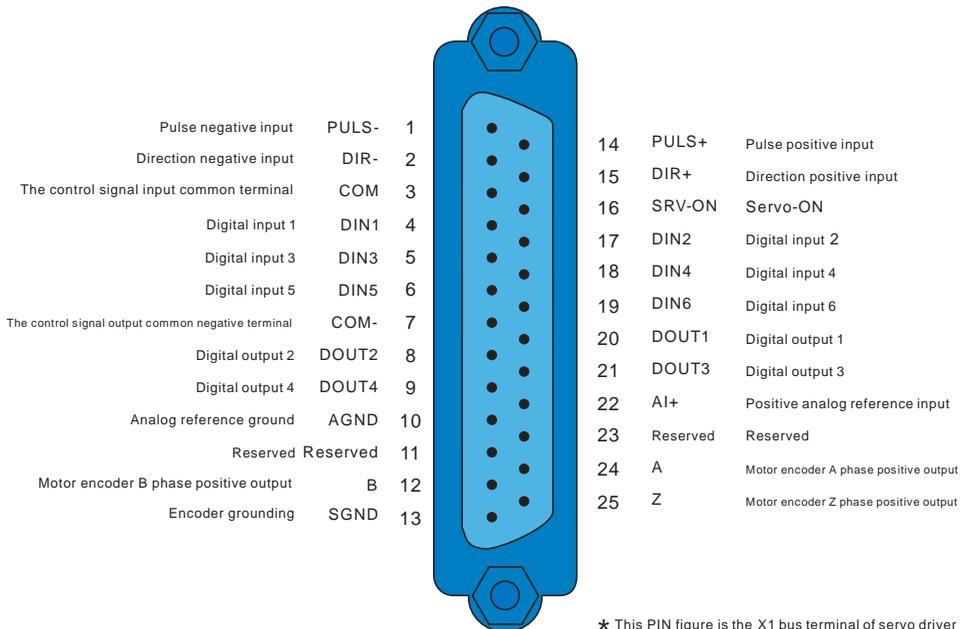
★ This PIN figure is the X1 bus terminal of servo driver
