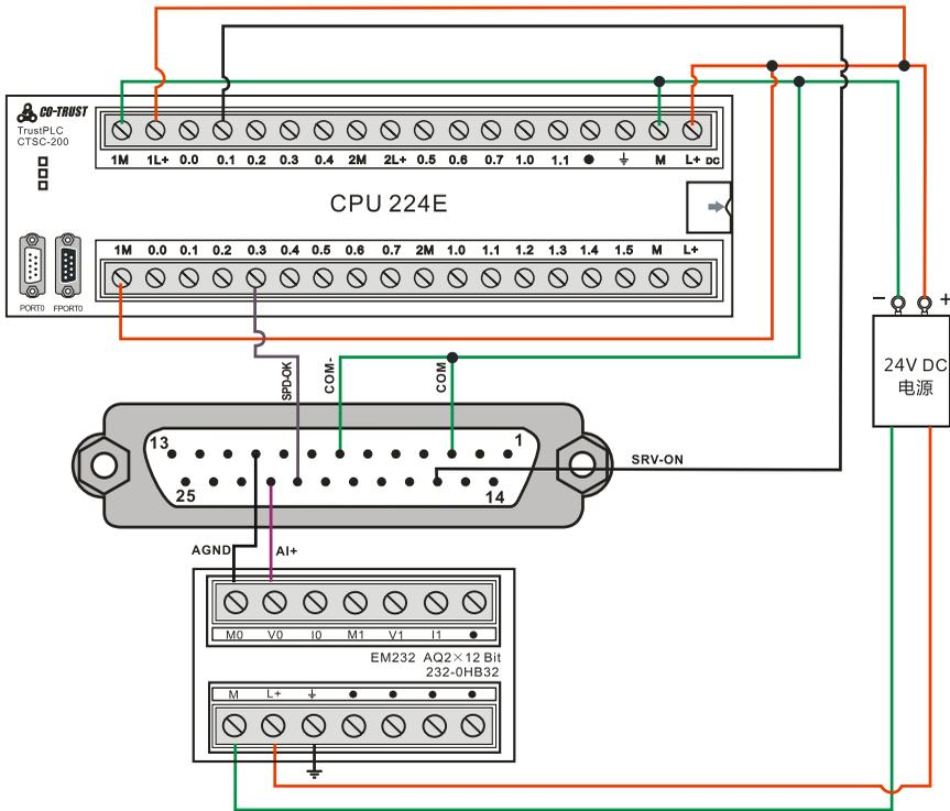
8.2.3 Application Example of External torque control mode
