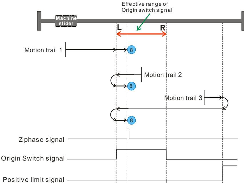
As seen above, machine is moving to the positive limit switch, Z-phase signal is located at right of left edge of the original point signal, which is within the range of original switch.
