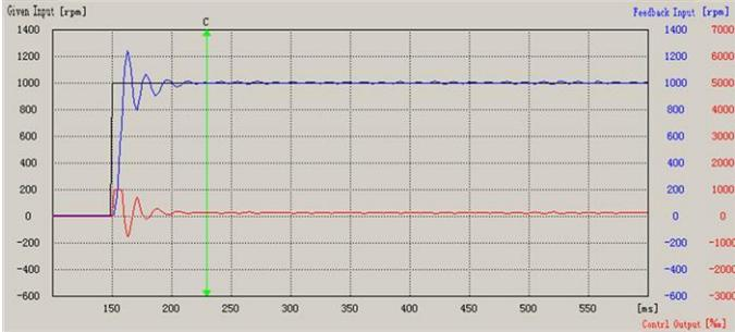
Figure 9.1 The speed loop curve at high gain of speed loop
