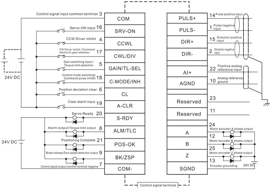
1、Single-ended drive mode, please do not connect external resistance while using 5V power supply.
