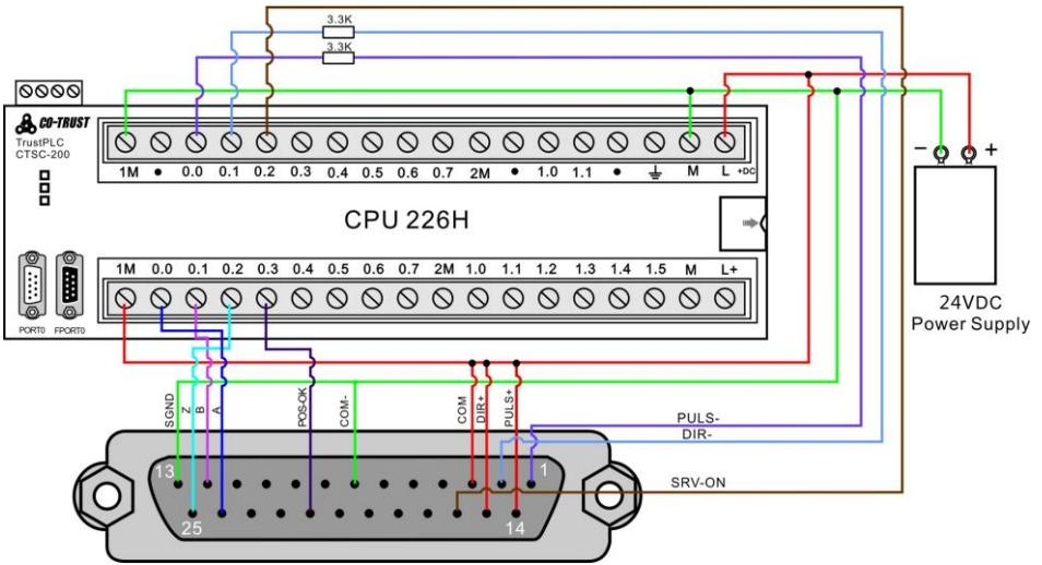
If PLC (such as Siemens PLC) or upper computer uses PNP output, the connection refers to following diagram:
