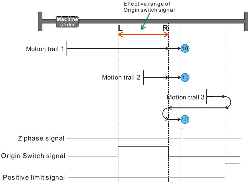
As seen above, machine is moving to the positive limit switch, Z-phase signal is located at right of right edge of the original point signal, which is out of the range of original switch.
