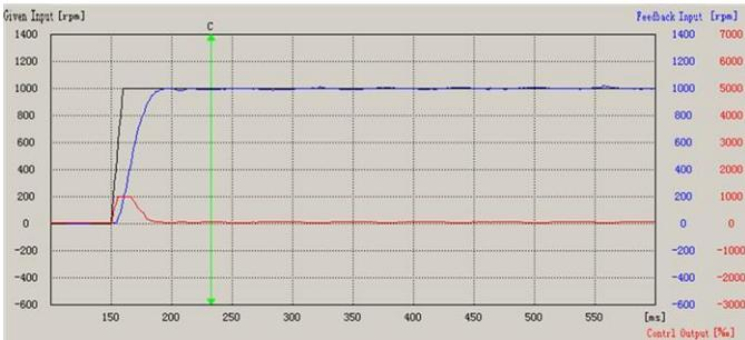
Figure 9.3 The speed loop curve of proper speed loop gain
