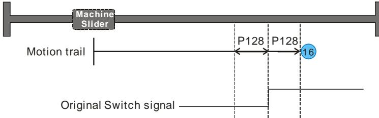
When P128 is positive value, the machine slider would finish the given position of P128 in positive direction.
