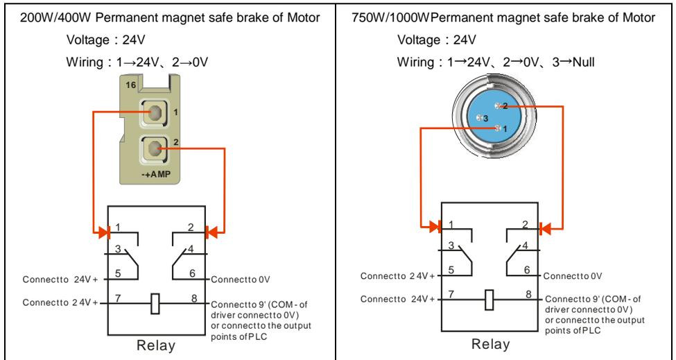
**<Note>** Connect the control terminal of brake resistance via relay (Control terminal: DC24V, load capacity is greater than or equal to 1A), and connect a Schottky diode in parallel at the control terminal of relay (Diode type is recommended as 1N4148, Package: DO-35 glass package, instrumented).
