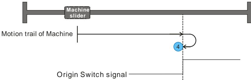
Original switch is located in the positive direction of the machine. The machine is moving in the direction of original switch, it would slow to a suspend while the original switch is detected, then exist from the original switch and turn back to search the falling edge of original switch, after that it would mark the falling edge as the original point, and the motor stop immediately.
