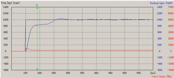
Figure 9.2 The speed loop curve at low gain of speed loop
