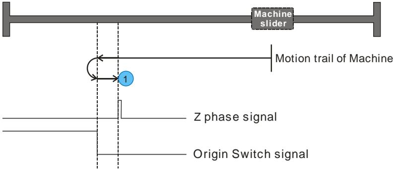
Original switch is located in the negative direction of the machine. The machine is moving in the direction of original switch, it would suspend while original switch is detected, then exist from the original switch and turn back to search the next Z-phase signal of motor, after that the servo would mark the first Z-phase signal as the original point, and the motor stop immediately.
