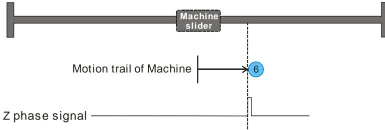
After received the homing command, the motor is moving in positive direction, and it would record the next Z-phase signal as the original point.
