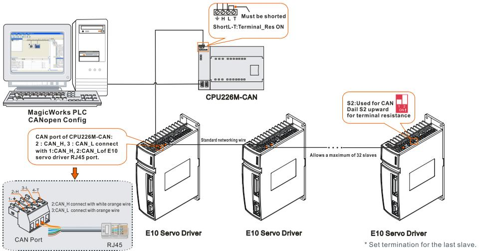
**<Note>** Be sure to set terminal resistance for CPU226M-CAN and the last slave device.
