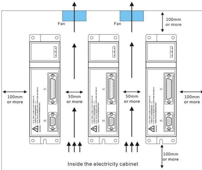
Figure 3.2 Installation intervals for one or more servo drivers
