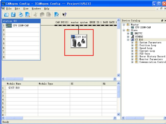
④ Expand CT E10 node from Device Catalog, and select the desired params to start communication position control for E10 Servo. The params selected for E10 are described as follows:
