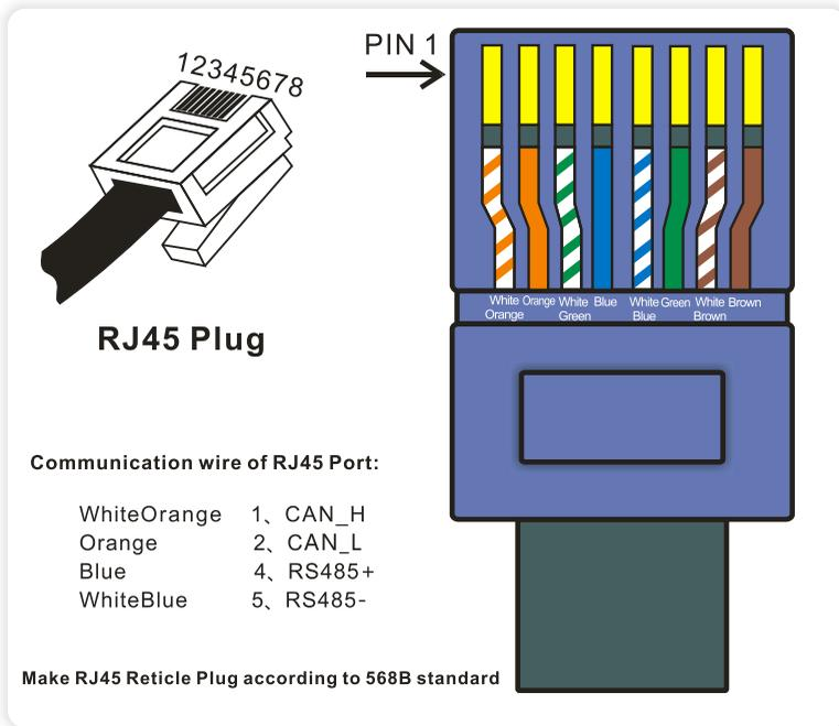
Figure 4.7 Reticle plug schematic diagram
