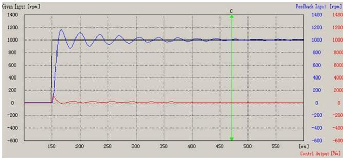
Figure 9.4 The speed loop curve at low speed loop integration
