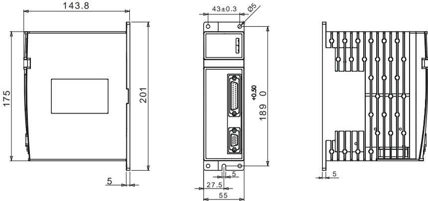
Figure 3.1 Base plate installation method of Servo driver
