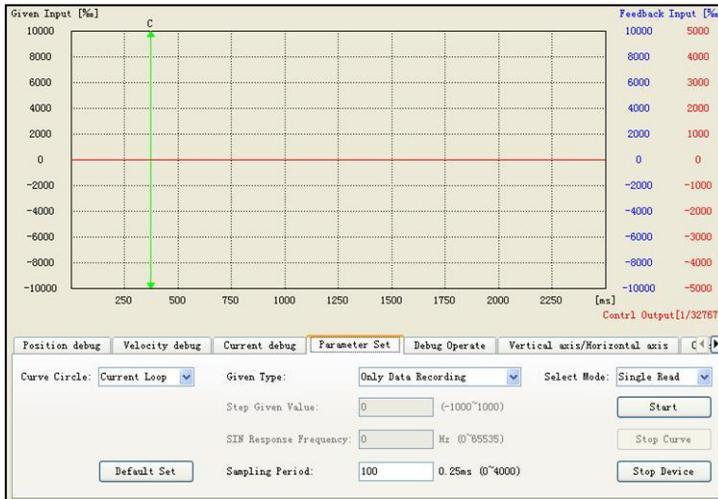
We can check the Current loop (or Speed Loop, or Position Loop) by clicking the pull-down box of "Curve Circle", and might also single Read or Cycle Monitor by selecting the pull-down box of "Select Mode". Clicking "Start" button to start the motor, then begin to sample data and draw the curve. Clicking "Stop Curve" button to stop the record of curve but not stall the motor, you might stop the motor by clicking "Stop Device" button.
