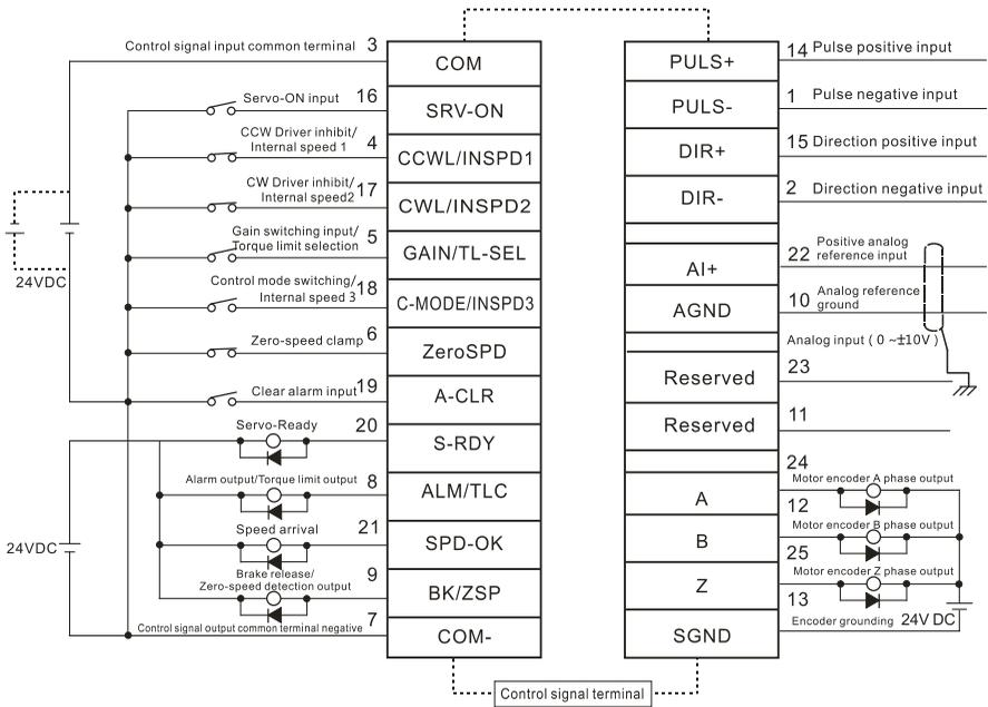
1. The voltage of control signal power between COM+ and COM- is 12 to 24V; Make the lower limit voltage of power supply between COM+ and this signal as 12V or more in order to ensure the control signal input is valid. (When you use contact inputs, use the dedicated switches and relays for micro current to avoid contact failure)
