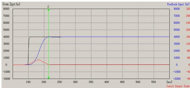
Figure 9.7 The position loop curve of proper position loop gain
