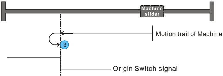
Original switch is located in the negative direction of the machine. The machine is moving in the direction of original switch, it would slow to a suspend while the original switch is detected, then exist from the original switch and turn back to search the falling edge of original switch, after that it would mark the falling edge as the original point, and the motor stop immediately.
