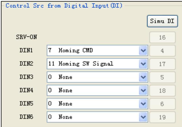
Stop “Simu DI”, the signal of DIN1~DIN6 would be inputted by external pins.
