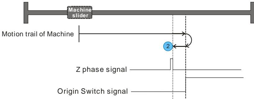
Original switch is located in the positive direction of the machine. The machine is moving in the direction of original switch, it would suspend while original switch is detected, then exist from the original switch and turn back to search the next Z-phase signal of motor, after that the servo would mark the first Z-phase signal as the original point, and the motor stop immediately.
