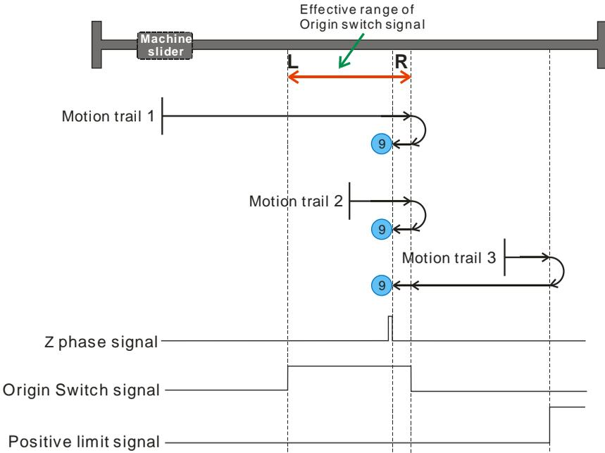
As seen above, machine is moving to the positive limit switch, Z-phase signal is located at left of right edge of the original point signal, which is within the range of original switch.
