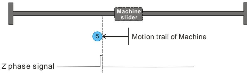
After received the homing command, the motor is moving in negative direction, and it would record the next Z-phase signal as the original point.
