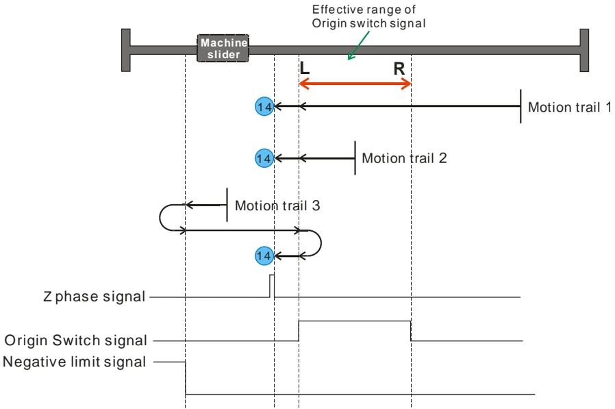
As seen above, machine is moving to the negative limit switch, Z-phase signal is located at left of left edge of the original point signal, which is out of the range of original switch.
