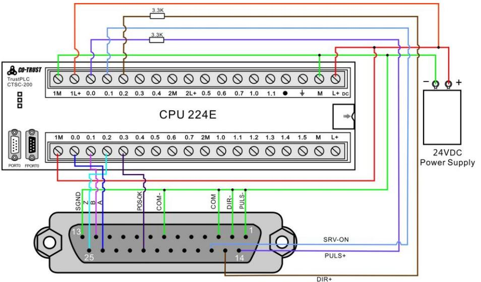
**Step 5:** After the wiring is completed, the controller enables the servo driver and sends out pulse command, the pulse indicator begins to twinkle, and the motor starts to rotate. Please check the monitor parameters (R235 \ R202) while motor stalls.
