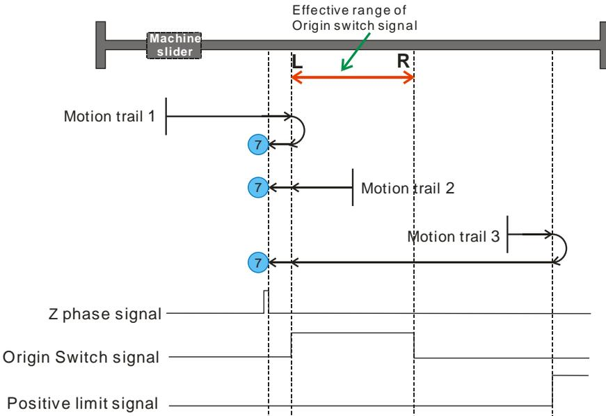
As seen above, machine is moving to the positive limit switch, Z-phase signal is located at left of left edge of the original point signal, which is out of the range of original switch.
