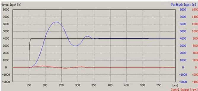
Figure 9.5 The position loop curve at high gain of position loop
